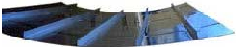
Figure 1 Typical model found in the aerospace industry with a panel riveted to a doubler panel
