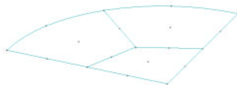
Figure 8: Corner Crack With 3 Elements
