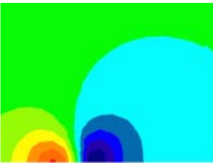
Underwater electric potential 50m below the ship
