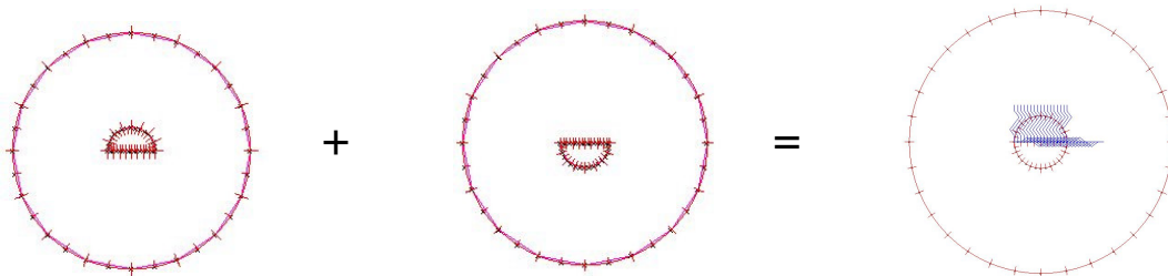
Fig. 2: Rivet half engaged with skin (left), with doubler (centre) and assembled rivet (right).
