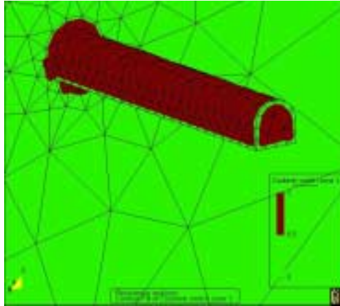
Figure 1: Mohr-Coulomb criterion result near the crossing fracture zone in the first model without EDZ.
