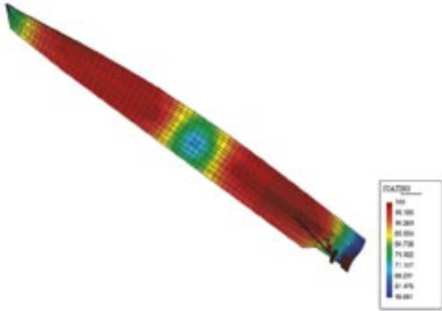
Figure 13 Predicted areas of damage on the vessel using the inverse analysis
