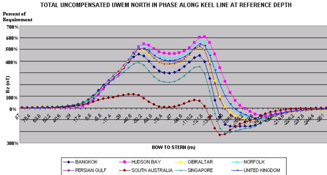
**Figure 6 Total Uncompensated In-Phase UM Signature Along Keel Line, For Various Worldwide Locations, North Heading**
