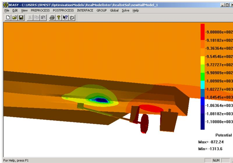
Figure 15: Distribution of potential over the surface.
