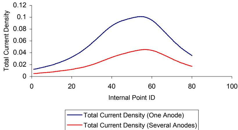
Figure 19: Resultant-current density along sampling line
