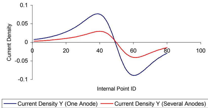
Figure 17: y(vertical)-current density along sampling line
