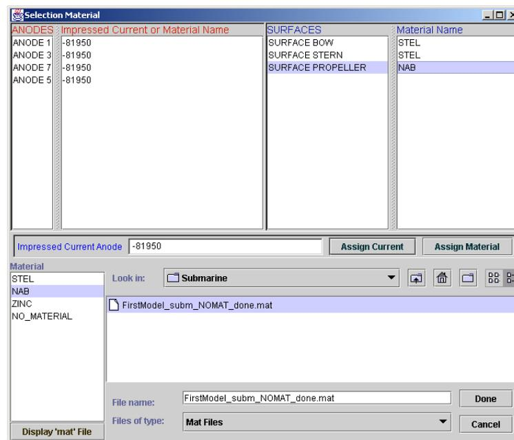
Figure 4 View of the design visual user interface where the properties of the anodes and the construction materials can be selected and quickly changed
