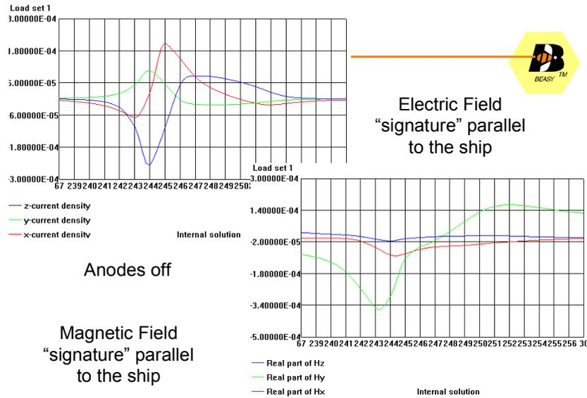
Figure 5 UEP and CRM example signatures computed using the same model
