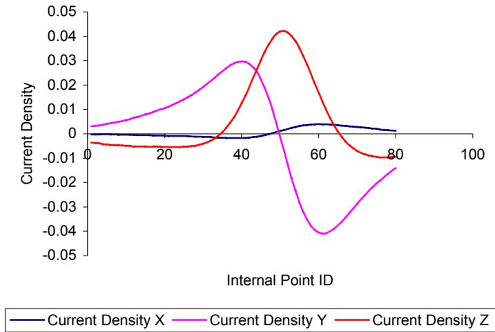
Figure 14: Current Density components along sampling line for optimised solution 7 anodes.
