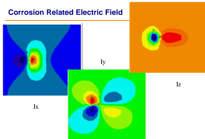
Figure 4 UEP Field at mid depth, no anodes
