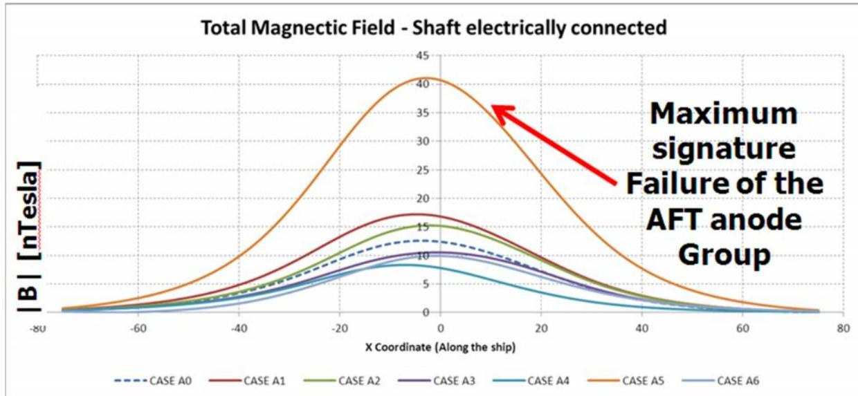
Figure 6 Predicted magnetic signatures for different failure scenarios assuming the shaft was grounded
