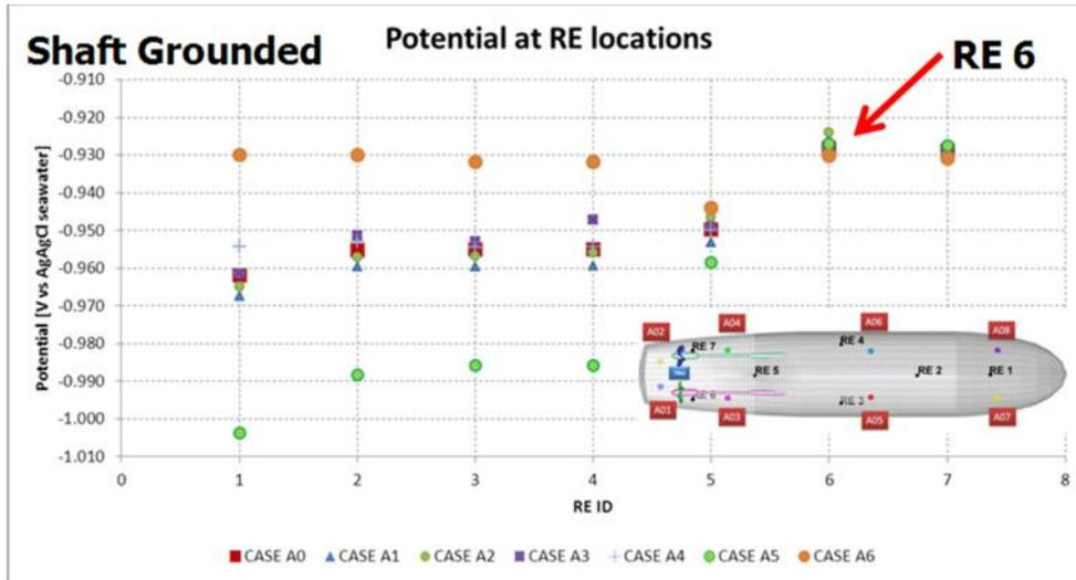
Figure 4 Predicted potentials at the reference electrodes (X axis)
