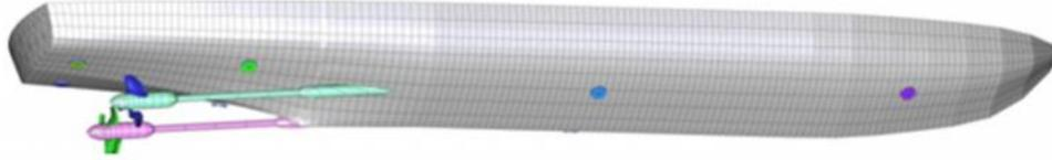
Figure 1 Simulation model of a ship showing the computational mesh used to represent the shape and properties of the vessel
