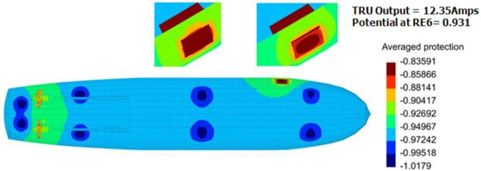
Figure 11 Predicted hull potentials with hull penetration assuming the shaft is grounded
