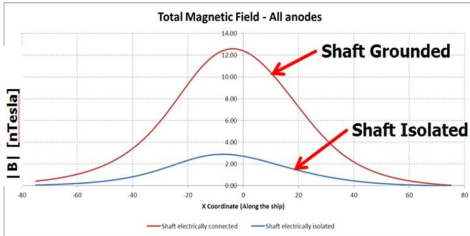
Figure 8 Predicted variation in the total magnetic field for different shaft grounding assumptions
