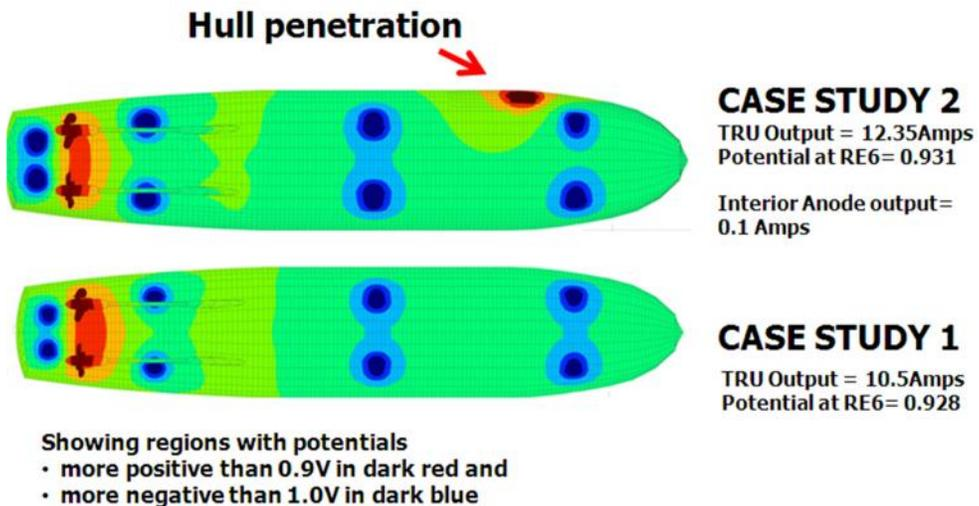
Figure 13 Predicted hull potentials with and without hull penetration assuming the shaft is grounded and all anodes are active
