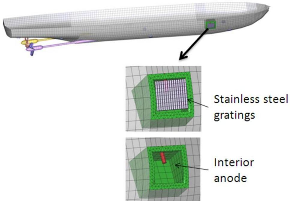
Figure 9 Hull penetration with stainless steel grating and internal anode
