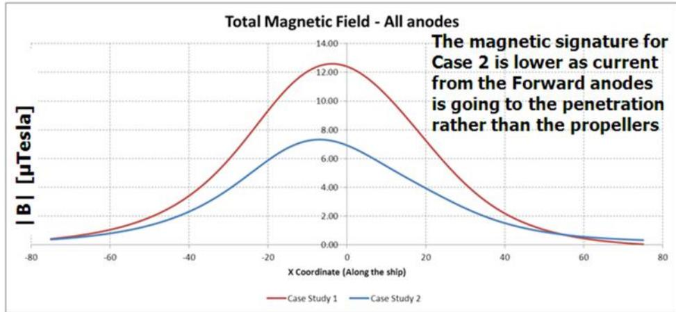
Figure 14 Predicted magnetic signature with and without the hull penetration assuming the shaft is grounded and all anodes are active
