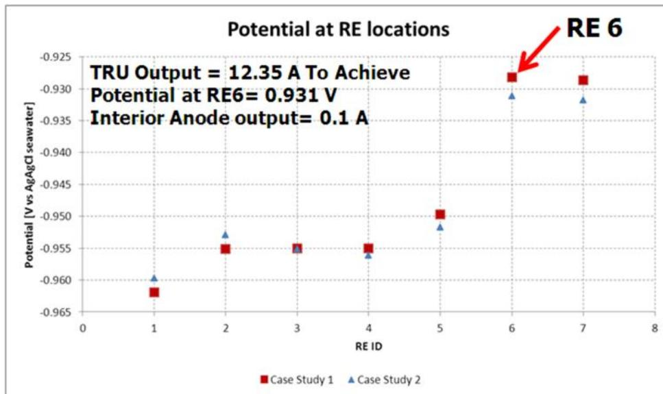
Figure 10 Predicted potentials at re locations with hull penetration with the assumption that the shaft is grounded and all anodes are active
