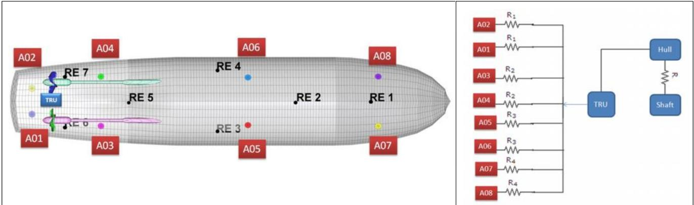
Figure 2 Ship anode and reference electrode locations. The electrical connections are shown assuming the TRU is located in the stern
